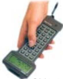
Fully integrated RFID read/write functionality for MIFARE.
