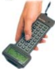
Fully integrated RFID read/write functionality for Tag-it and I-Code smart labels.
