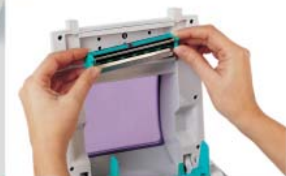
▼ Tool-less printhead replacement
